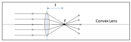
Figure 2: Light paths through a convex lens
