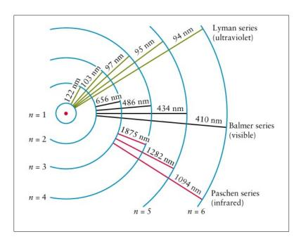
Figure 2: Energy levels in a hydrogen atom
