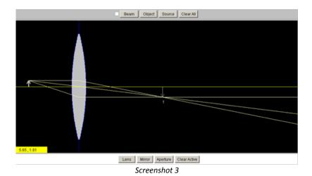
Question 6: Notice that the real image formed by the objective lens (labeled "1") is not located at the focal point of the lens. This is because the object is relatively close to the lens. Select the lens and slide it all the way to the right and back. Does the position of the real image change with respect to the focal point as the lens-object
