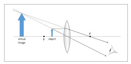
Figure 5: A convex lens as a magnifying glass
