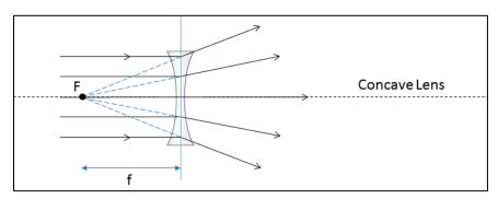
Figure 3: Light paths through a concave lens
