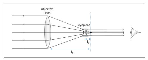
Figure 7: A concave lens as a telescope's eyepiece
