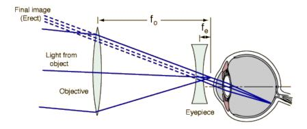
Figure 1: Image formation in Galileo's telescope.
